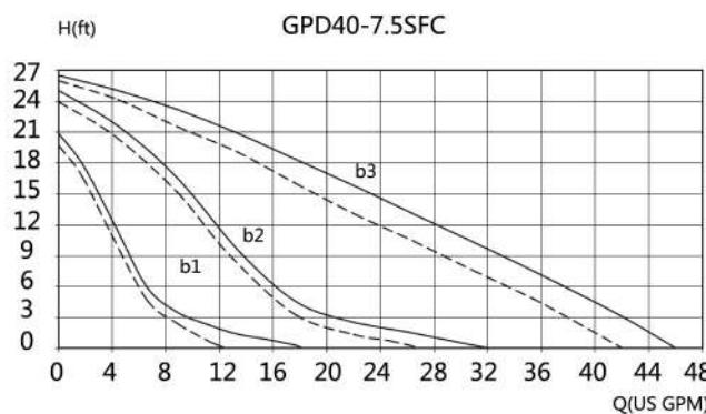
"— without check valve, "----"with check valve
