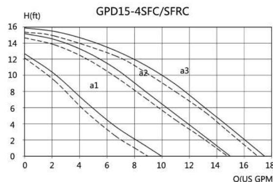
"—" without check valve, "----"with check valve
