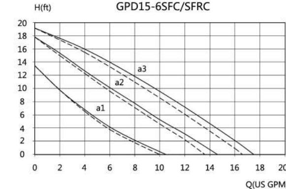
"—" without check valve, "----"with check valve
